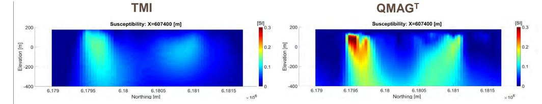
**Technolmaging** has developed a regularized inversion scheme employing a focusing stabilizer and Gramian constraints to invert FTMG data. Inversion runs for both susceptibility and components of the full magnetization vector.
